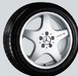
17 STYLE I AMG 5-spoke wheel 7.5 J x 17 ET 37 · 225/45 R17 B6 603 1005 High-sheen rim flange; not for SLK 350 or SLK 55 AMG
