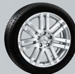
17 7-TWIN-SPOKE WHEEL 7.5 J x 17 ET 47 · 225/45 R17 A204 401 0502 Titanium silver finish
