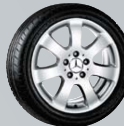
17 7-SPOKE WHEEL 7.5 J x 17 ET 56 · 235/65 R17 B6 647 4247* Titanium silver finish; not in conjunction with R 500
