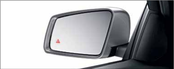
Passive Blind Spot Assist is available as part of the optional Driving Assistance Package.
