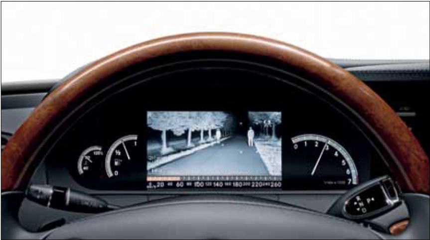
Night View Assist utilizes infrared technology to assist during night time driving.
