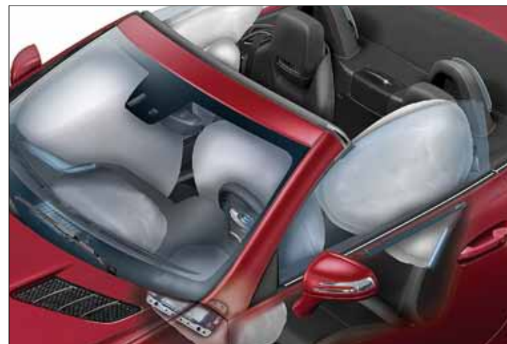
Head airbags reduce the risk of injury by providing additional support in the event of a collision 1,3 .
