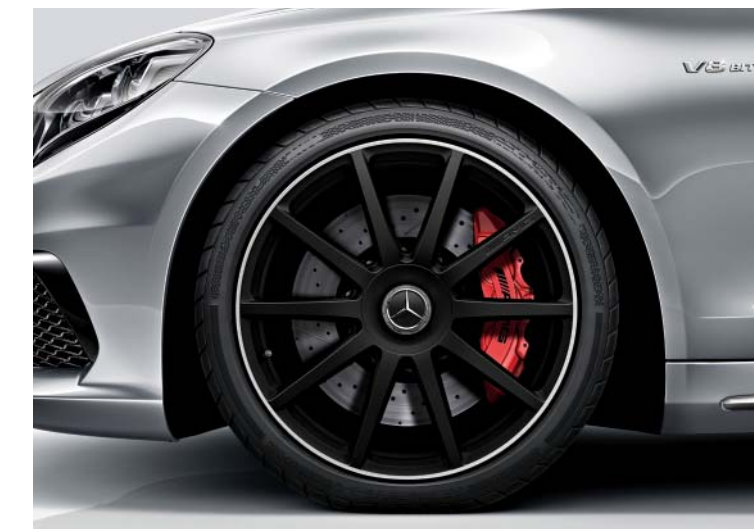
20" AMG 10-spoke forged alloy wheels in matte black with red painted brake calipers. 1
