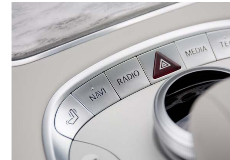
Central operating unit with COMAND controller.
