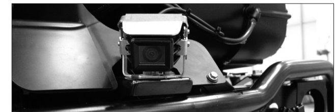
Roof-mounted windscreen wiper system and front camera
