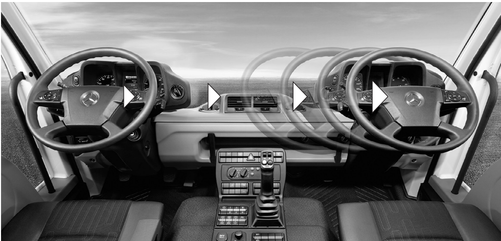
Interior view with VarioPilot® transferable steering
