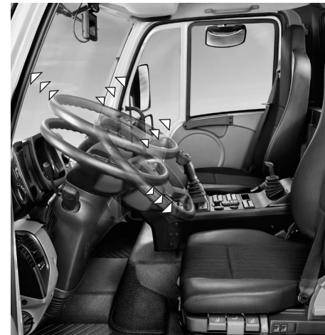
Steering column adjustable in height and tilt
