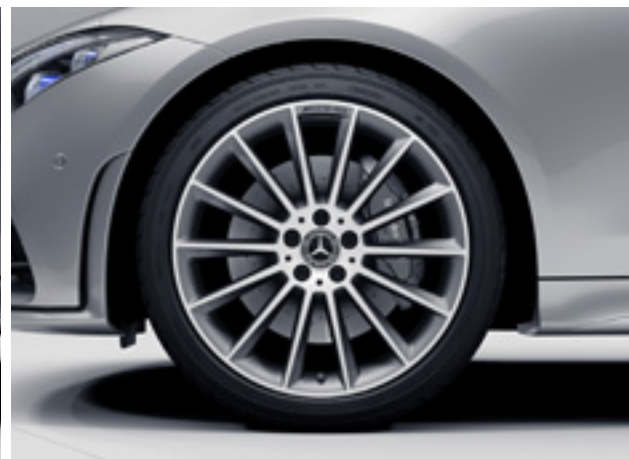
RVO 20" alloy wheels (4) – multi-spoke design front: 245/35 tyres; rear: 275/30 run-flat tyres
