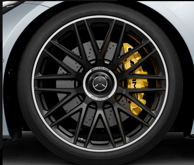
RWE 21" AMG forged wheels - 10-twin-spoke design, painted matt black with a high-sheen rim flange, 295/30 (front) and 305/30 (rear) R21 tyres
